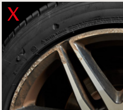
Excessive damage to wheels
